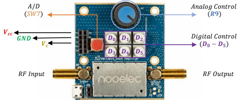
\* The Variable Gain Amplifier allows for 3 different power options (USB, Pin Header and Bias-Tee). At any given time not more than one option should be used.
