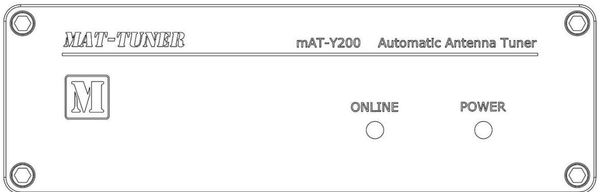
**ONLINE:**Status indication. Lights up to indicate that the tuner is online, off-indicates that the tuner is bypass.
