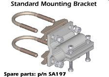
Materials: extruded aluminum Hardware: stainless & zinc plated steel Dimensions: 80 x 76 x 65 mm
