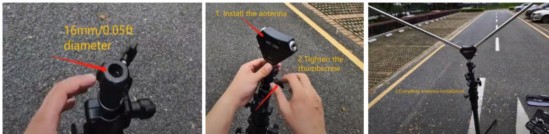
3. Loosen the thumbscrew and extend each section to the desired height. Re-clamp each section and verify that it is secure and will not allow the tube to slide down.
