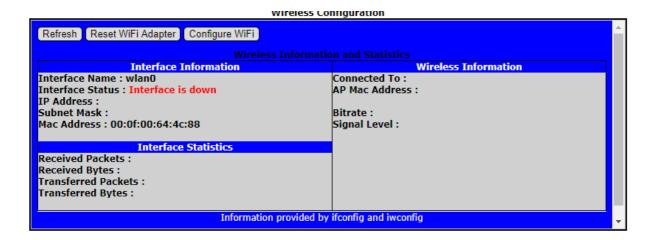
To add your wifi, simply click on configure wifi. Make sure the wifi-dongle is connected to the radio, this screen will only be shown when this dongle is available.
