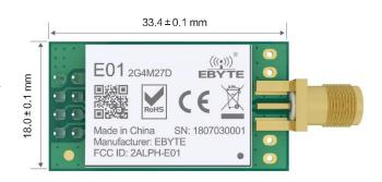
that the maximum transmit power reaches 500mW while the receiving sensitivity improves for three times to -99dBm. The products have been greatly improved when there is no PA and LNA in design.
