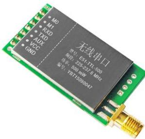
E51-TTL-500 is a 500mW wireless transceiver module(UART), with transparent transmission, operates at 225-237.6MHz z(default 230MHz),narrow-band transmission &TTL level
