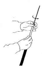
The desired frequency can be adjusted by the FRP element length. With longer element size, the frequency will move to lower side and shorter length move the frequency to higher level. The frequency change per 1cm length is 110kHz.
