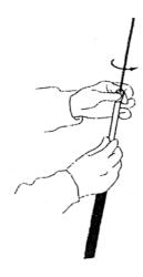
The desired frequency can be adjusted by the FRP element length. With longer element size, the frequency will move to lower side and shorter length move the frequency to higher level. The frequency change per 1cm length is 56kHz.
