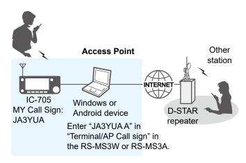
Before using the DV Gateway function, you have to set up a network.
