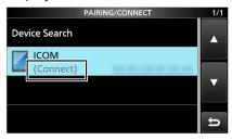
**NOTE:** If you cannot connect, check that the same CI-V address is set between the transceiver and the RS-MS1A.
