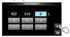
Returns to the DR screen, and "Link to Reflector" and entered reflector is displayed in "TO."
