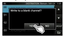
The operating data is entered in the selected channel. "FROM" and "TO" names are automatically entered as the Memory name. (Up to 16 alphanumeric characters.)
