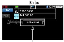
"GPS ALARM" pops up on the screen and the alarm sounds 3 times.
