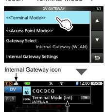
"Ext" is displayed when using the External Gateway function.
