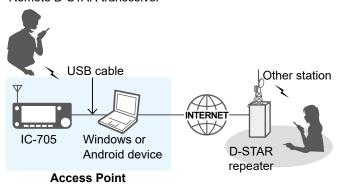
\* Any model as long as the transceiver is D-STAR capable. Only one D-STAR transceiver can access the Access Point at the same time.
