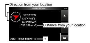
\* When a name is not entered in the GPS Memory channel, date and time are displayed instead of the name. In the QUICK MENU screen, you can change the GPS Memory or GPS Alarm in the GPS POSITION screen. (p. 12-6)
