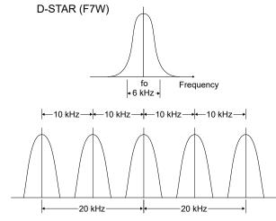
D-STAR occupies 10 kHz. The sound quality is good, even though the bandwidth is narrow.
