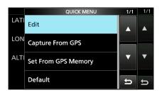
**TIP:** When you select "Capture From GPS" or "Set From GPS Memory," you can capture the position from the GPS, or set the Object's position from the GPS memory.
