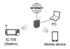
When "Connection Type" is set to "Access Point (Connect to Phone, PC)," you can directly connect your PC or mobile device to the transceiver for:
