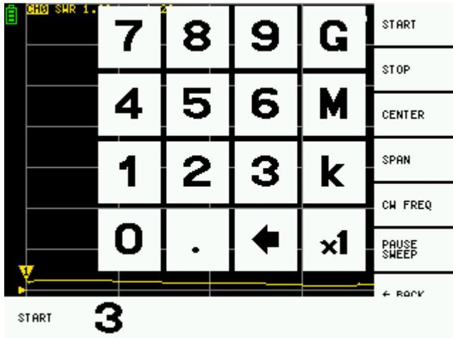
On the keypad screen enter **3** then tap on **M** (for MHz) in the keypad unit column.
