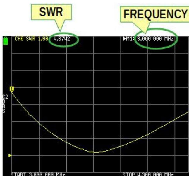
Now, we have yellow trace on the screen. It is a graph of SWR versus frequency. Notice the yellow marker, the yellow triangle with number 1. The position of the marker on the trace reveals the frequency and the SWR at that frequency. In Figure 102, the cursor is at 3 MHz and the SWR at that frequency is 1: 4.67.
