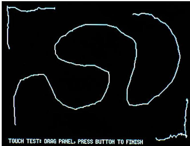
To verify the accuracy of the touch screen calibration, select **CONFIG - TOUCH TEST**. Draw on the screen with the stylus. The touch screen is of resistive technology and needs the right amount of stylus pressure to work properly. If necessary, repeat the touch screen calibration.
