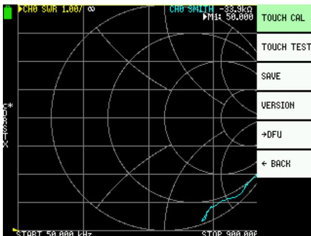
Slide multifunction switch to the left several times to highlight the **TOUCH CAL** menu option. Now, press the multifunction switch to execute the selected command.
