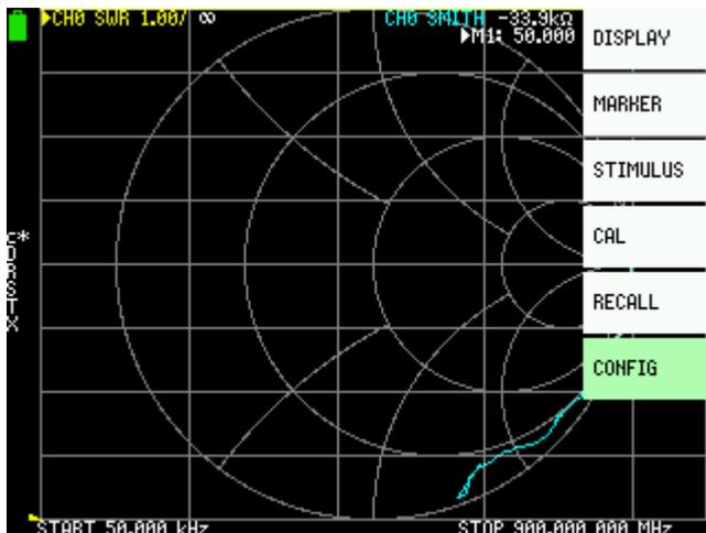
As the touch screen is not yet calibrated, press the multifunction switch. This will open the menu as in Figure 11.
