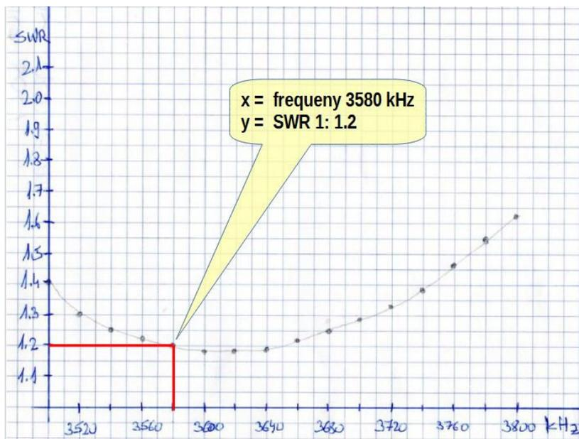
A picture is worth a thousand words! On the drawn graph, we see the SWR of our antenna on the whole band at first glance. For example, if we are interested in SWR at a frequency of 3580 kHz, we draw a vertical line from the 3580 kHz label on the x-axis to the graph. From this point of intersection, we draw a horizontal line to the y-axis and read the SWR from the y-axis.
