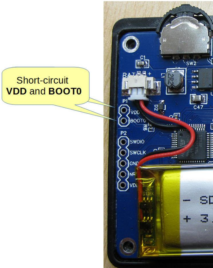
To get back into DFU mode, all you have to do is boot the NanoVNA whilst you have the two VDD and BOOT0 points on the printed circuit board shorted together (Fig. 77).
