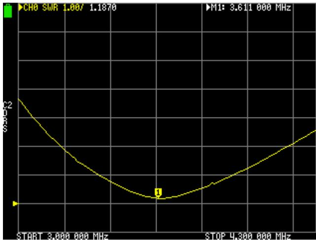
The best SWR is where the graph is closest to the reference line (Fig 103). The marker can be moved by sliding multifunction switch or by dragging with the stylus.
