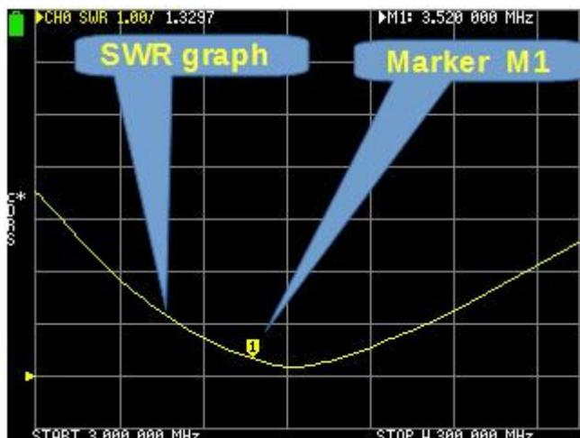
The above procedure took us some time. NanoVNA can produce a similar graph (a trace in the VNA jargon) on the screen in a second (Fig. 18). In the NanoVNA we set up the frequency span, choose which trace we want to see on the screen and connect the antenna. The rest is NanoVNA's job.
