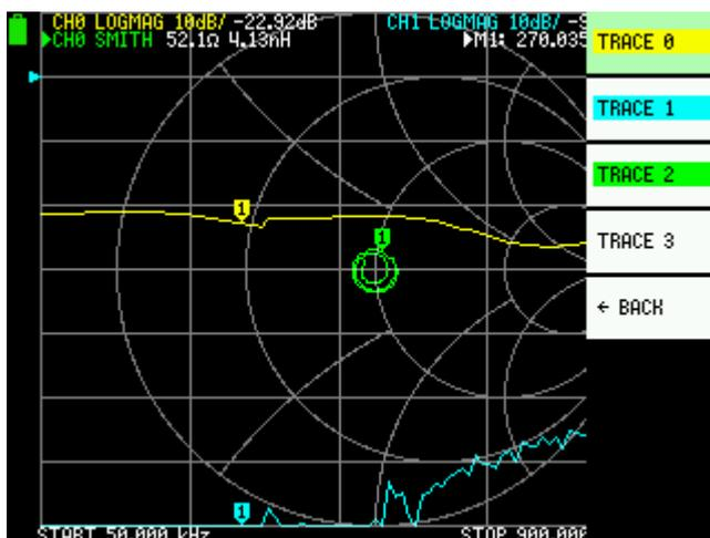
The NanoVNA can display up to four traces, **TRACE 0**, **TRACE 1**, **TRACE 2** and **TRACE 3**. As we can see from Figure 27, traces number 0, 1 and 2 are highlighted, (the background color of the trace names is highlighted in the same color as the color of the trace). This indicates the traces that NanoVNA will display. The background color of TRACE 3 is white – it is not used at the moment.
