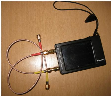
I use a short flexible cable such as the RG174 to relieve the mechanical stress on the SMA connector on my NanoVNA (Fig 37). This means that the calibration must be done at the end of that cable, not on the NanoVNA.
