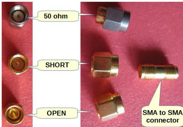
Calibrate the NanoVNA with the calibration standards that came with the device: OPEN, SHORT and 50 ohm (Fig 36).
