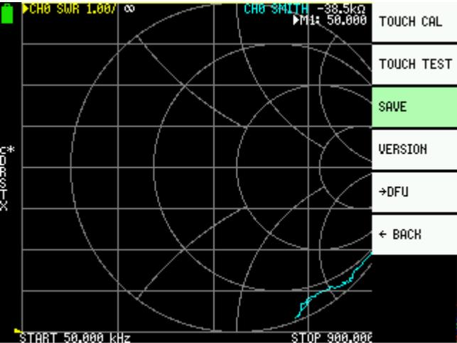
Slide multifunction switch to the right to highlight the **SAVE** menu option, and then press the multifunction switch to execute the **SAVE** command.
