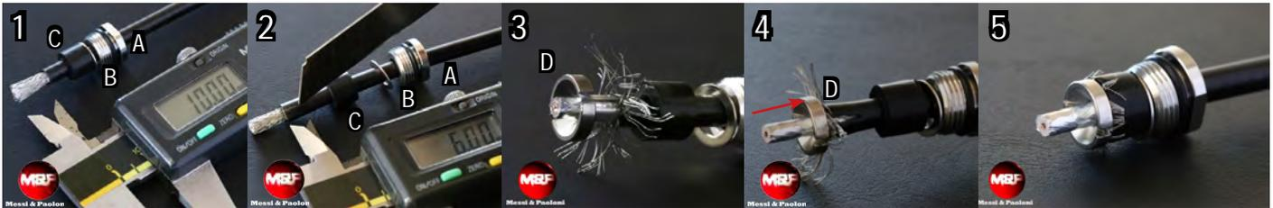
1 Make a circular cut on the black PVC outer jacket at the indicated length shown in the caliber (in mm). Subsequently remove it.
