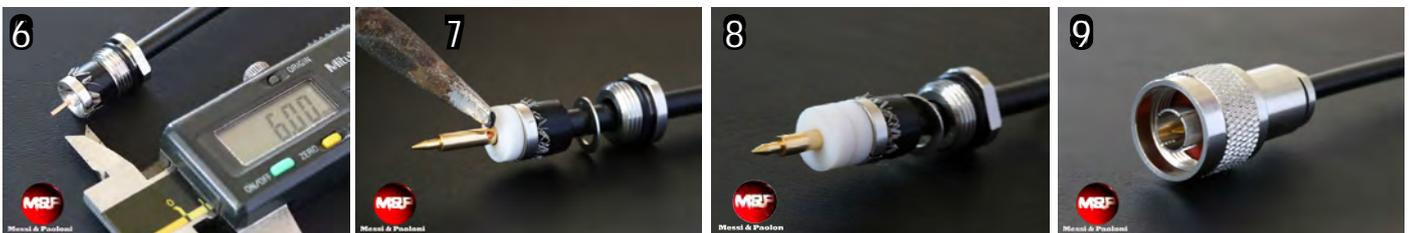
6 Cut and remove the tape and dielectric for a length as shown in the picture (in mm).
