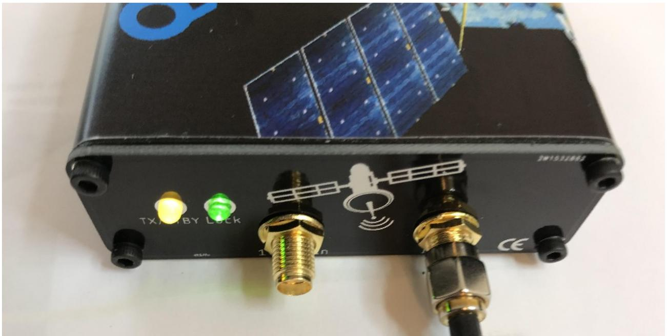
*Fig 4 TX mode, TX/STBY led is Orange*
