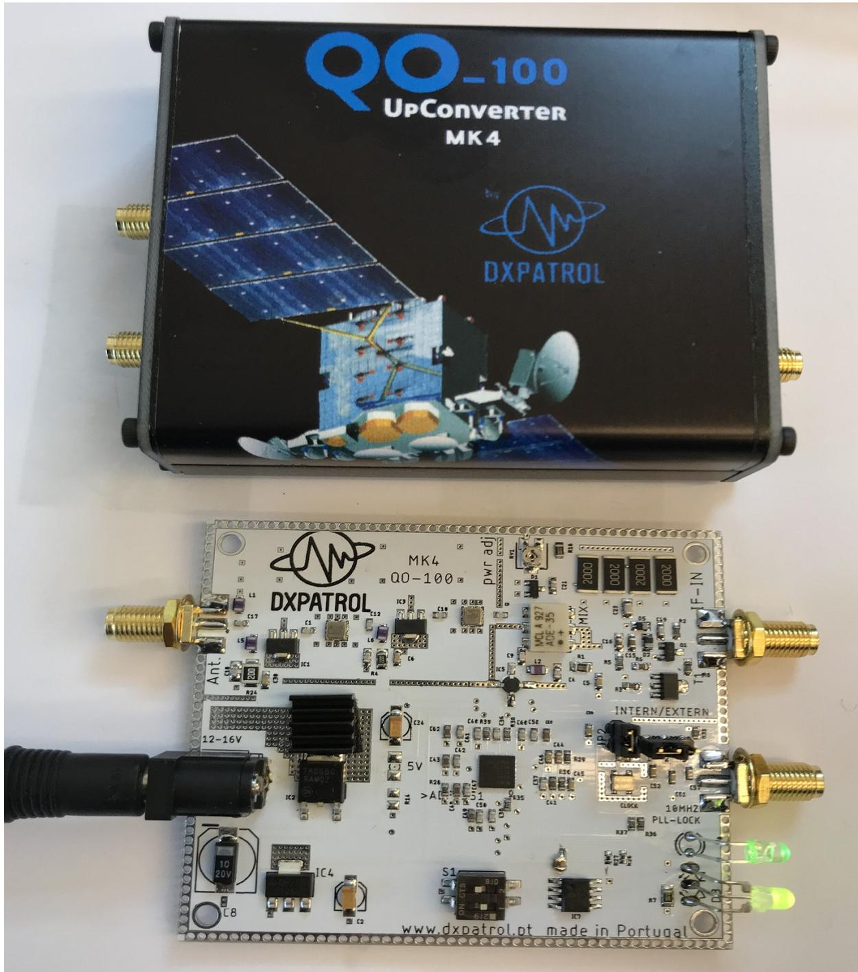
fig 1, Upconverter full assembled PCB
