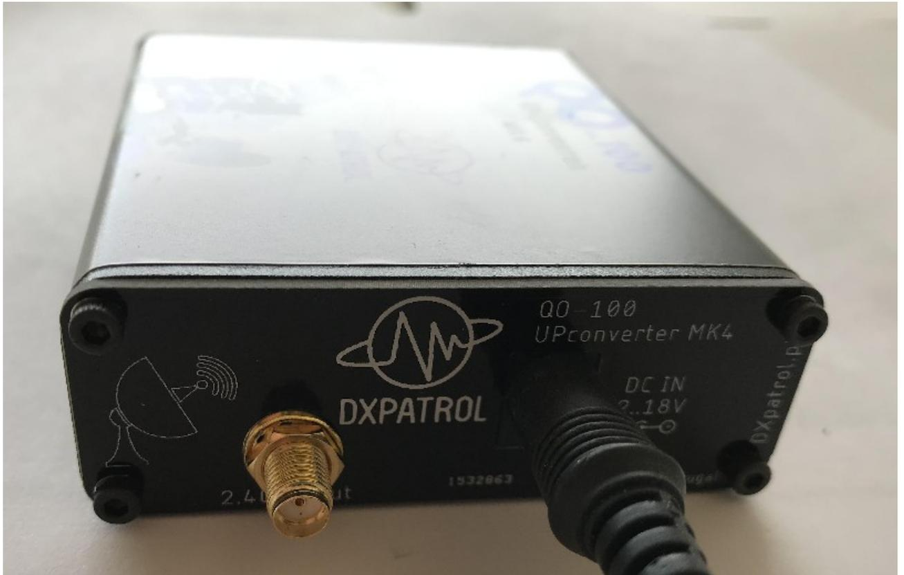
*Fig 2 DC connection, ( positive to center pin)*
