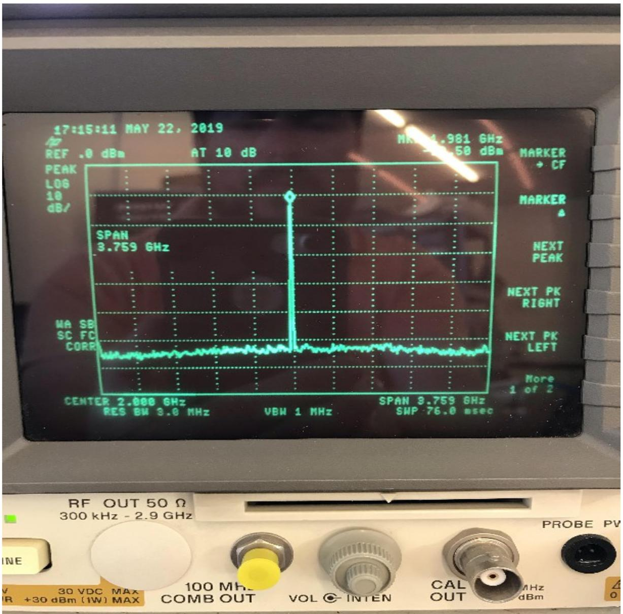
Fig 5 spectrum view 3,8Ghz span (local oscillator)
